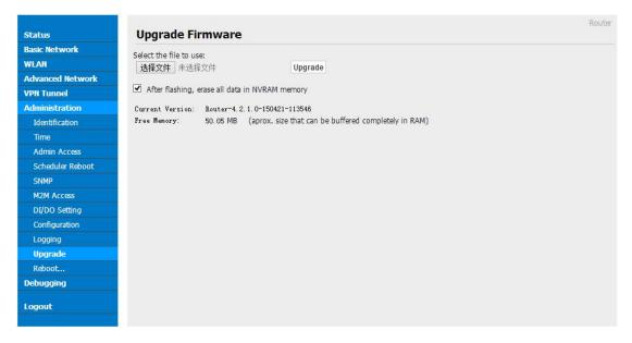
Figure 3-32 Firmware Upgrade GUI
